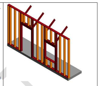
74 B2010.05-LOD-350 Exterior Wall (Cold-Form Metal Framing)
