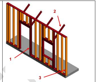
97 C1010.05-LOD-350 Interior Wall (Cold-Form Metal Framing)
