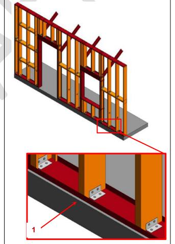
98 C1010.05-LOD-400 Interior Wall (Cold-Form Metal Framing)
